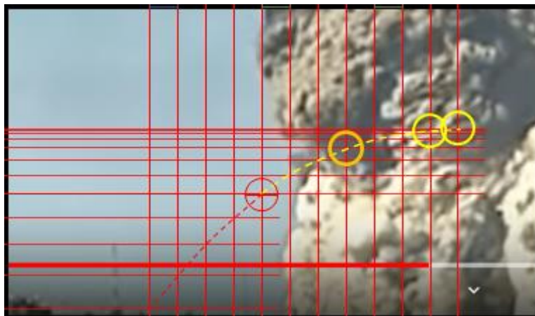
Figure 20: Implied location 1.00 second before initial observation (red circle is the location of the initial observation; orange circle is the imputed location 1.00 second earlier).
